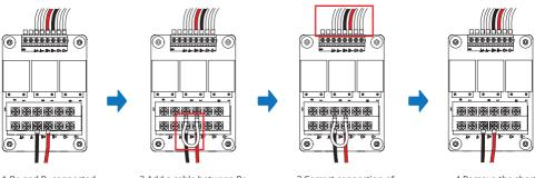
1.B+ and B- connected reversed
