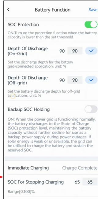
Through battery function settings, you can set parameters for battery connected in the system.
