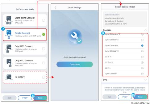
**Step 8**:Set the working mode based on actual needs. Tap **Next** to set the Working Mode. For some models, after the working mode configuration is completed, it will automatically enter the CT/meter self-test state. At this time, the inverter will temporarily disconnect from the grid and then automatically reconnect.
