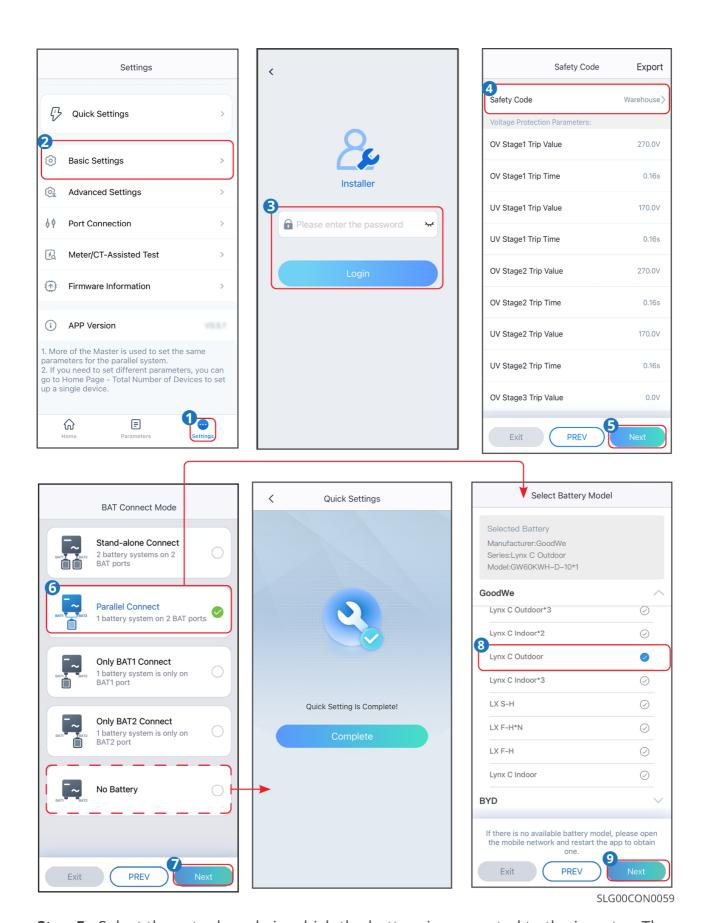
Step 5: Select the actual mode in which the battery is connected to the inverter. The
