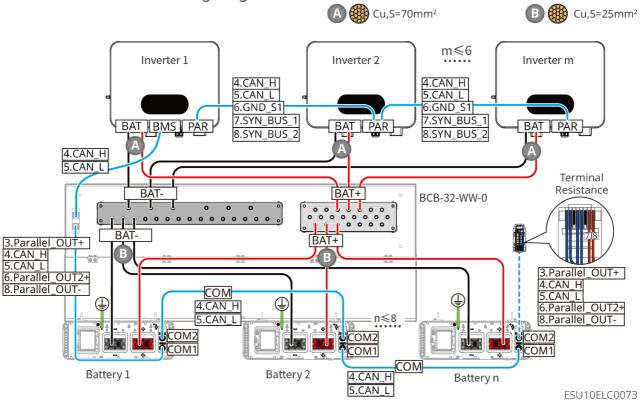
LX U5.0-30: When the battery quantity is less than or equal to 15, and the busbar BCB-33-WW-0 is used, the wiring diagram is as follows:
