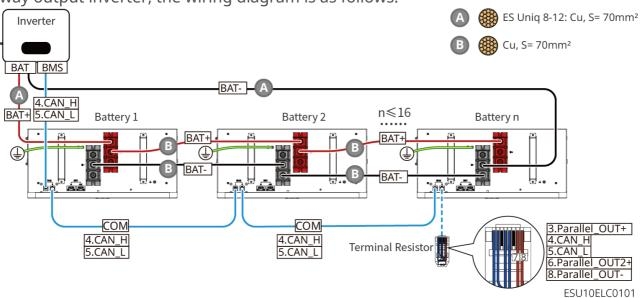
GW14.3-BAT-LV-G10: When the number of batteries is less than or equal to 16 and a busbar (BCB-32-WW-0, Current≤ 720A) is used to connect 1-way output inverter, the wiring diagram is as follows:
