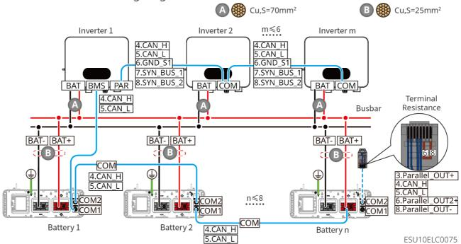
LX U5.0-30: When the battery quantity is larger than 8, and a third-party busbar is used, the wiring diagram is as follows:
