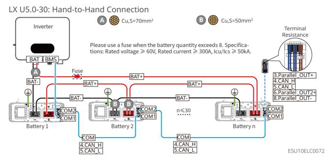
LX U5.0-30: When the battery quantity is less than or equal to 6, and the busbar BCB-22-WW-0 is used, the wiring diagram is as follows:
