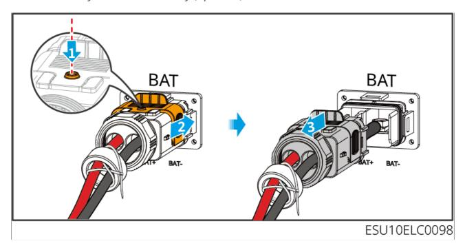
Battery power cable manufacturing (LX A5.0-10 and LX A5.0-30)
