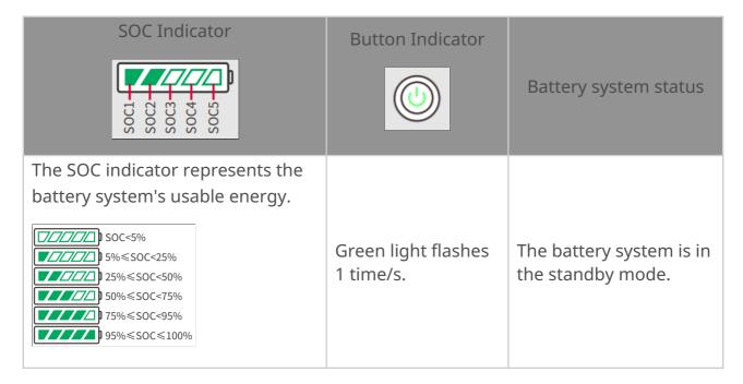
Maximum SOC indicator flashes 1 time/s, other green lights always on. • When 25% ≤ SOC < 50%, SOC2 flashes. • When 25% ≤ SOC < 50%, SOC2 The battery system is Green light is on. flashes. working normally. • When 25% ≤ SOC < 50%, SOC2 flashes. • When 25% ≤ SOC < 50%, SOC2 flashes. • When 95% ≤ SOC < 100%, SOC5 flashes.
