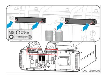
Step 2: Installing the plastic cover
