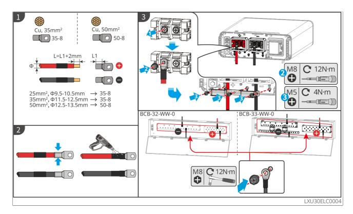
Battery power cable manufacturing (GW14.3-BAT-LV-G10)
