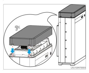
• Use a flathead screwdriver to gently pry up the two clips on one side, and then remove the plastic top cover.
