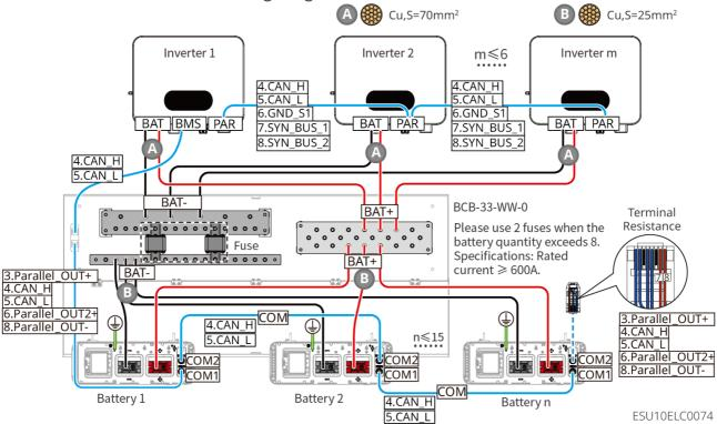
LX U5.0-30: When the battery quantity is less than or equal to 8, and a third-party busbar is used, the wiring diagram is as follows:
