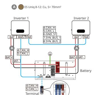
GW14.3-BAT-LV-G10: When the battery is in hand-to-hand connection with a single 1-way output inverter, the wiring diagram is as follows:
